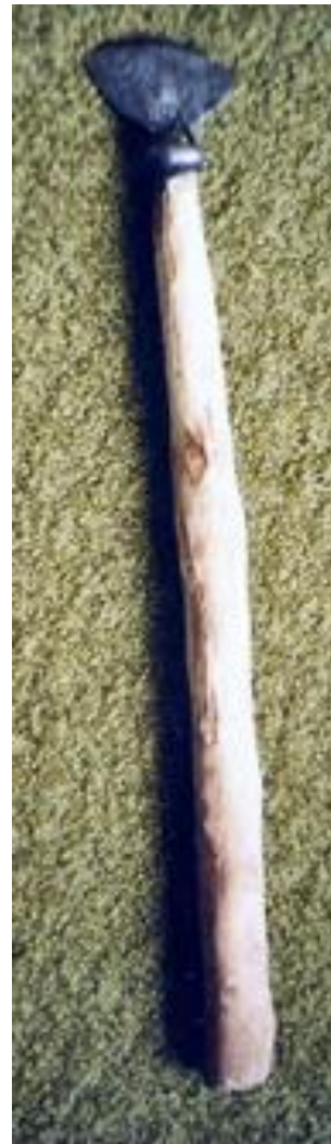
2 • tool for softening leather (a mieli-blade fixed to a straight handle). Ba pa mieli a tag gbangka. They take a mieli to soften leather.
